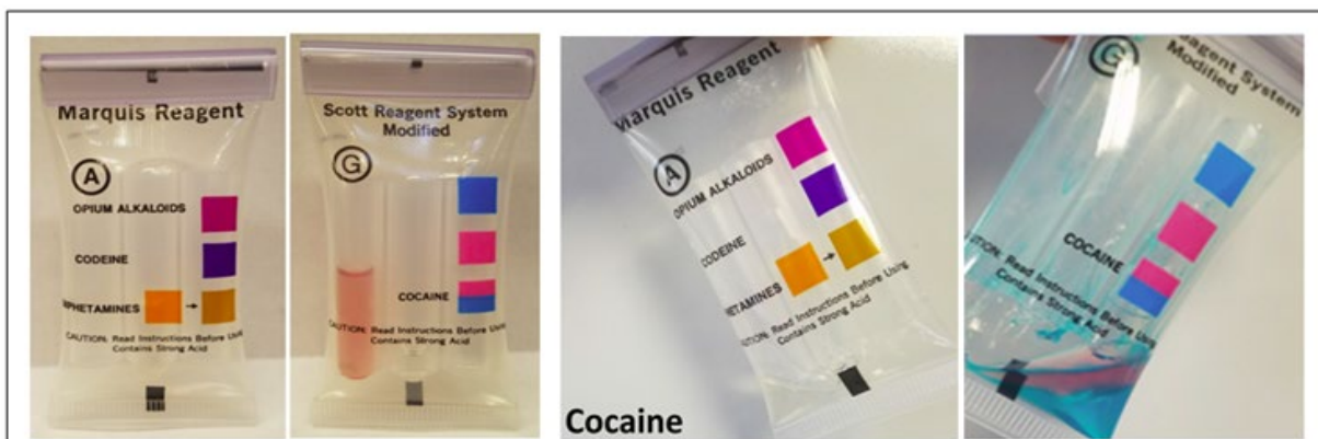
Figure 2: From left to right, NIK-A and NIK-G straight out of the box, and then NIK-A after testing cocaine giving a colorless solution so no color change, and then NIK-G after testing cocaine to give pink layer over blue layer, resulting in a positive presumptive test for cocaine.
