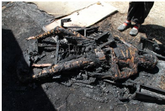
Figure 23: Test 6B: After fire, left arm crossed across body, legs splayed, feet disarticulated. Position of body changed by collapse of chair beneath
