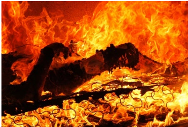
Figure 2: Test 1: At 16min, the right arm is raising at the elbow and the legs are flexing upward due to flexing of the knees
