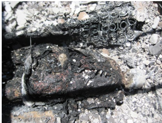
Figure 37: Test 12: This adult male body was in a supine position on the innerspring mattress during a demonstration fire in a furnished cubicle. During the fire, the mattress collapsed and the body ended up in a supine position on the floor adjacent to the bed
