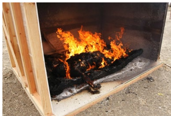
Figure 9: Test 2: At 2hrs:15min, the fire is localized on the body and the pool fire beneath it. The right arm has collapsed outward
