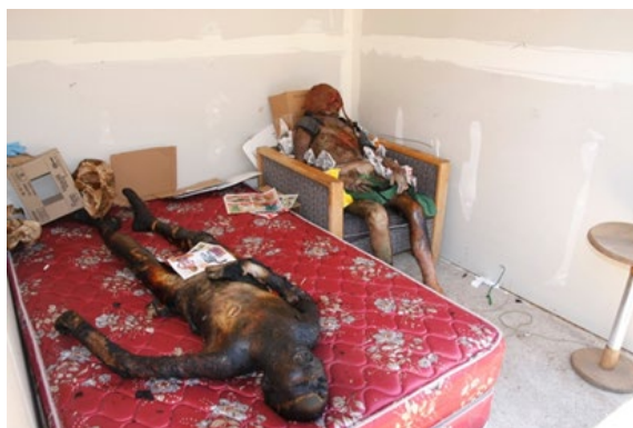
Figure 11: Test 3: Open cubicle fire with two bodies. One body (previously exposed to a low intensity fire) on bed, other slumped in chair. Fire started in paper trash between body and chair. Fire went to flashover at about 7min, post-flashover burning for 13 more minutes (total fire duration was 20 min.)
