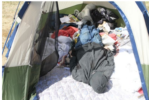
Figure 35: Test 11: Tent fire. Adult female body clothed in sweatshirt and pants supine on a spring mattress. Ignition by cigarette on cotton bedding (at feet). Arms at sides, legs straight and together. Duration of flaming fire 20min
