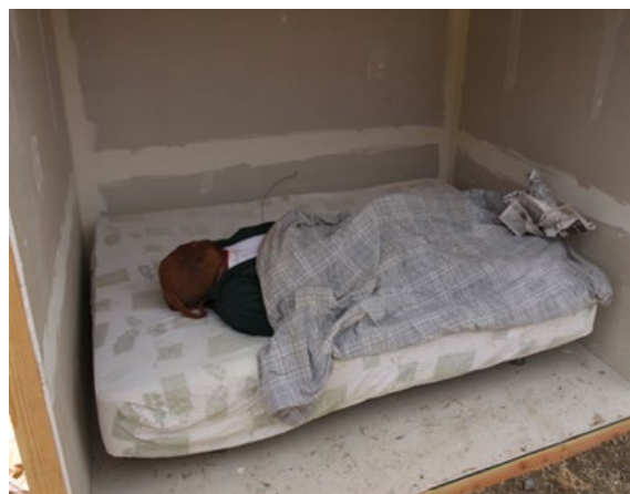
Figure 6: Test 2: Sustained fire in bed. Body of elderly male adult in supine position on modern box spring, dressed in cotton sweatshirt and pants and covered with a cotton blanket. Arms at sides, legs straight. Fire ignited in paper under edge of blanket at shoulder
