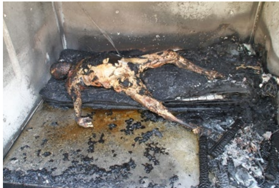
Figure 20: Test 6A: 15min. Subcutaneous fat exposed on torso and legs. Right arm extended out over edge of bed from shoulder. Right leg extended out over edge of bed. Left leg bent at knee. Intense fire on bed but did not proceed to flashover (carpet and wall still intact). Mattress collapse aiding movement towards edge
