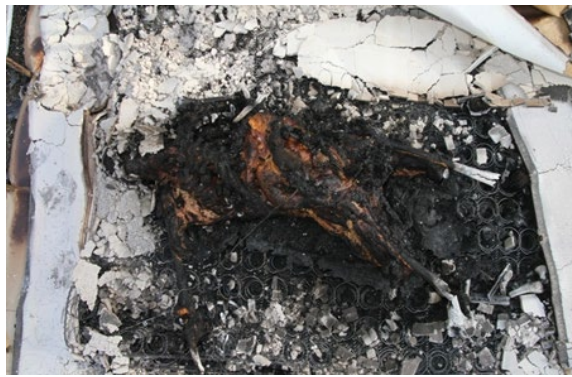
Figure 25: Test 7: 24min including post-flashover. Both arms extended well away from body and straightened. Legs spread but straight. Feet disarticulated
