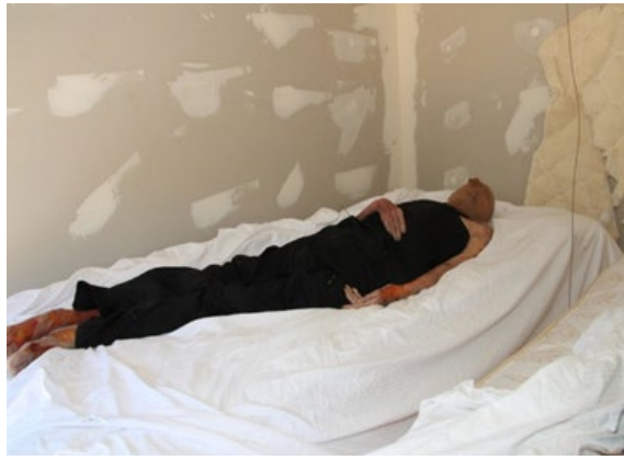
Figure 30: Test 9: Open cubicle – body on bed. Clothed, adult female body on top bunk. Ignition by open flame to bedclothes. Flashover within 1min
