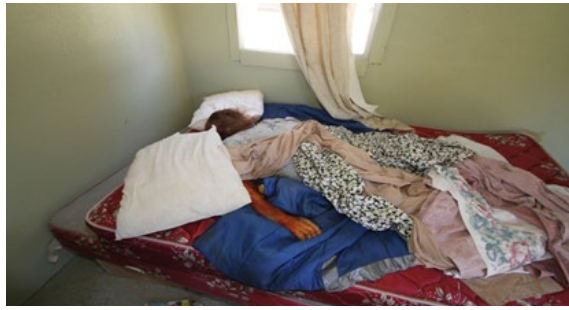
Figure 15: Test 4: Bed fire. Adult male body in supine position with legs straight and arms slightly extended. Fire started on bed. Total duration: 13min (including flashover)
