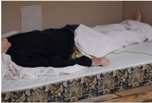
Figure 1: Test 1: Sustained fire on bed. Body of elderly male adult, dressed in cotton sweat shirt and pants on modern box spring, covered with cotton blanket. Body in supine position with legs extended straight and arms by sides. Fire ignited with open flame to paper at edge of blanket. Fire duration was 7 hrs (self-extinguished).
