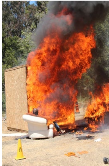
Figure 33: Test 10: Fire ignited on recliner by radiant heat from cubicle flashover fire at 1min. Head and arm rising and head turning towards the fire
