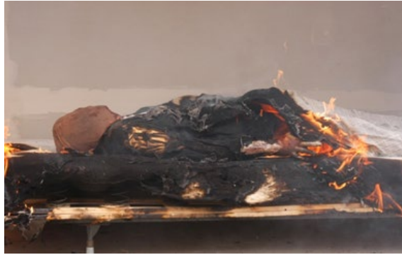
Figure 7: Test 2: At 1hr:16min, the modest fire in the box spring and blanket are causing the fingers of the right hand to flex downward (towards the heat)
