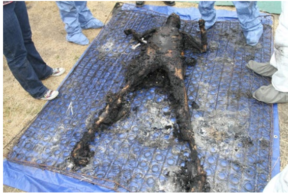
Figure 36: Test 11: After removal of tent and debris, body was left on inner spring mattress for removal. Arms flexed and rose. Legs straight but spread. Lower legs more badly damaged due to longer duration of fire in adjacent normal combustibles
