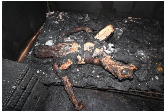
Figure 27: Test 8A: Duration 7.5min (3.5min post-flashover). Right arm extended out over edge of bed, right leg moved towards edge, both legs spread and flexed at knees
