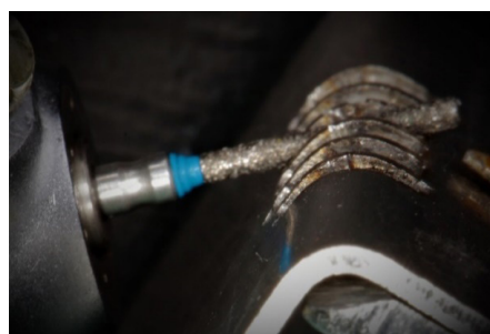
Figure-2 Skirt preparation through the guide
