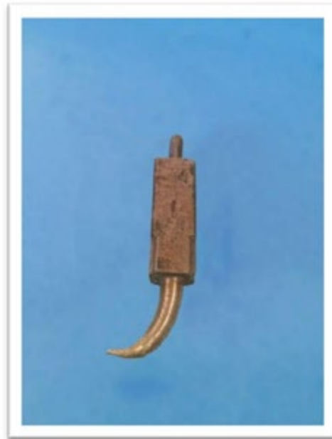
Figure 2: Specially made hook shaped attachment for tensile testing.
