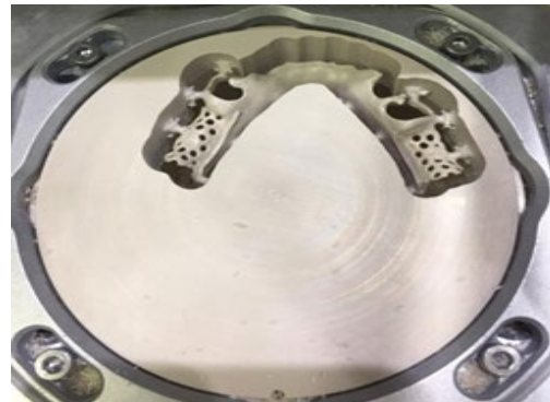
Figure 4: Milling of the framework from Juvora block
