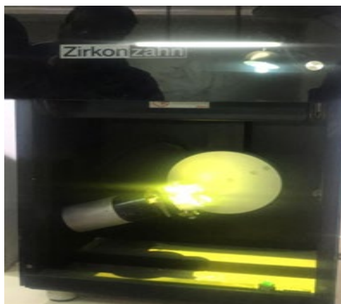
Figure 1: Optical scanning of the master cast
