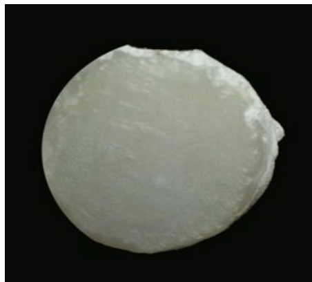
Fig 5: Translucent zirconia treated by cojet system showing cohesive layer within the resin cement (cohesive failure)
