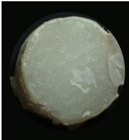
Fig 4: Translucent zirconia treated with hydrofluoric acid showing adhesive failure between resin and ceramic
